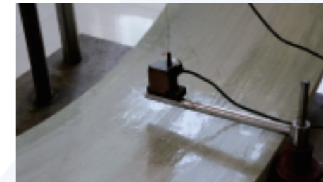
环刚度试验-测位移 Ring stiffness test - measured displacement
