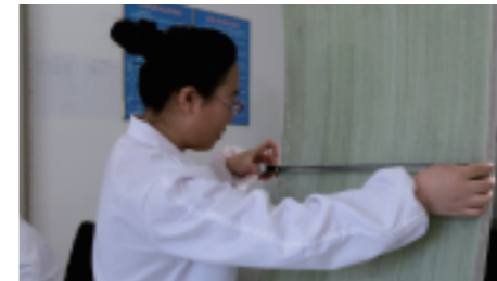
环刚度试验-测量试样宽度 Measure the sample width
